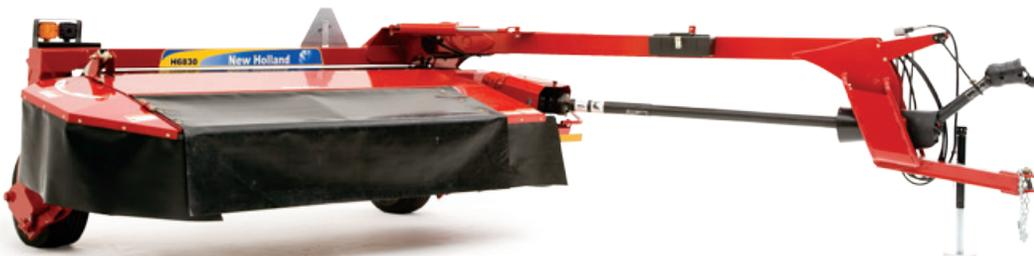
Tractor hook-up is easy. Simply drop in the pin, hook up the PTO and three hydraulic hoses. The primary PTO uses an 80-degree constant velocity joint that permits tight turning. If desired, your dealer can order an optional secondary PTO assembly with CV joint that allows you to steer the machine around field obstructions on-the-fly.
