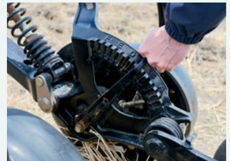
**Patented parallel link opener** gives the operator maximum productivity and seeding precision. The design allows for optimum seed placement combined with unmatched durability in a wide variety of soil conditions.
