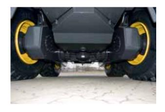
The rear tandem has been completely redesigned: **final reductions** are now located in the axle body while the brakes are positioned, for all models, in the hubs. A simple design which assures high durability.
