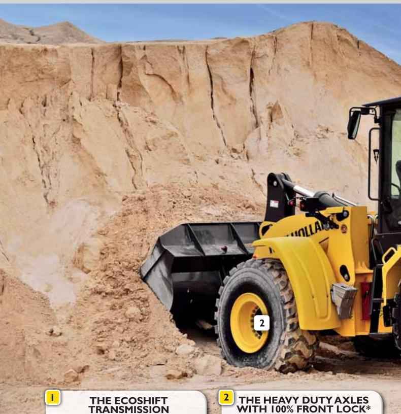
Type: ZF Power-Shift countershaft design whit four forward and three reverse speeds. Ecoshift uses engine de-rating to make each gearshift smoother and to optimize the pushing power of the torque converter. The Electronic Transmission System (ETS) include Inch declutching, Hold function, Kick-down and Downshift system allows the operator to dedicate 100% attention to the work cycles.
