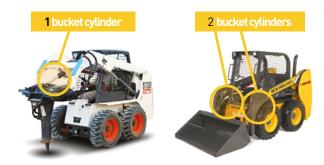
New Holland L213 has 2 bucket cylinders instead of 1: more digging efficiency and bucket balance
