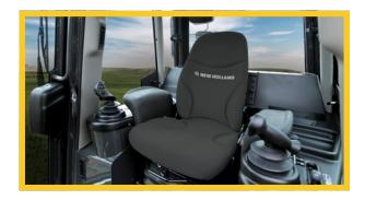
**5) COMFORT AND VISIBILITY for the perfect operator environment:** New Holland designed the operator compartment for more comfort and productivity. The cab is placed forward for accurate blade visibility and improved machine stability. Thanks to the two control joysticks with integrated advanced electronic functions, the driver can focus on the job and operate the machine with precision and less fatigue.
