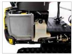
External sight gauges for easy checking of hydraulic and fuel levels. New filters and battery layout.
