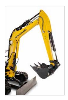
Auxiliary hydraulic functions (single or double acting) with pipings/hoses up to the dipper:
