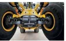
Note: On the W230C standard axles are available with open differential without autolock for flat, hard surfaces like tarmac.
