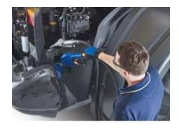
For security, the fuel tank and AdBlue tank are accessed only by raising the engine hood
