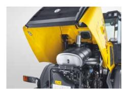
One piece engine hood features electric opening on W130 D,W150 D,W170 D and W190 D models
