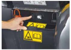
Hood raise switch, battery kill switch and remote battery terminals are grouped at the rear
