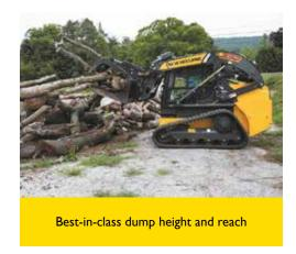
The vertical lift boom enables the operator to dump material much further and higher. Exceptional front reach makes it easy to load sided dump trucks or move materials around the warehouse.
