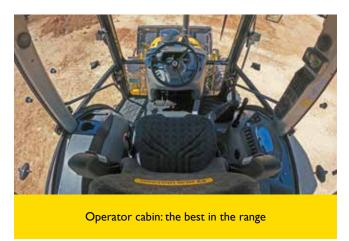
Climbing aboard a New Holland backhoe loader, you will find yourself in a comfortable, well-organized working environment with noise level as low as 77 dB(A). All loader controls are located on one joystick under the right hand. The fully adjustable luxury seat rotates 180 degrees to control the excavating equipment.
