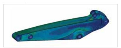
Booms and Arms have been redesigned using advanced CAD (Computer Aided Design) and FEM (Finite Elements Methodology) Systems to get higher strength **only** in those areas where stresses are concentrated.
