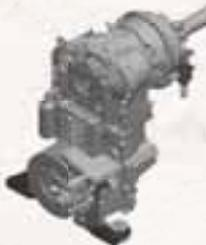
Type: ZF Power-Shift countershaft design with four forward and three reverse speeds. Ecoshift uses engine de-rating to make each gearshift smoother and to optimize the pushing power of the torque converter. The Electronic Transmission System (ETS) includes Inch declutching, Hold function, Kick-down and Downshift system allows the operator to dedicate 100% attention to the work cycles.
