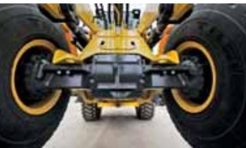
Note: For a limited investment, standard axles with limited slip differential are also available on the W170C and W190C. On the W230C standard axles are available with open differential without auto-lock, for flat, hard surfaces like tarmac.
