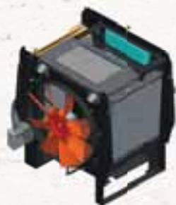
Most wheel loaders mount their radiators back to back. At New Holland we have mounted them to form a cooling module like a box. The benefit is better cooling, in the harshest of environments. In addition, with a programmable reversing fan as standard, cleaning radiators will become a thing of the past.
