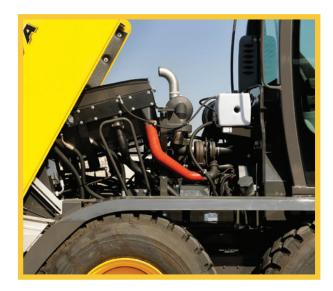
7) SERVICEABILITY – More uptime and durability as all major components are easily accessible at ground level, allowing for faster routine maintenance operations as well as quick intervention when needed. The engine and oil radiators can be easily checked thank to the new "flip-up" engine hood. The outward orientation of the central circle teeth, made of hardox steel, makes them easier to clean and better protected.
