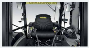
• High visibility is a key design priority—D Series loader backhoes deliver with extremely slim cab pillars, both front and rear
