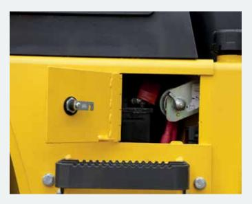
• Battery-disconnect and remote jump-start terminals are easily accessible
