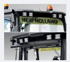
Up to 8 work lights, including roof-mounted side lights, are available
