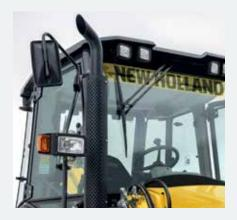
A-pillar-mounted exhaust offers a clear view of the loader
