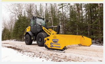
W70C and W80C axles can produce a top speed of up to 25 mph (40kph), able to drive from jobsite to jobsite in many cases eliminating the need for additional transportation with truck and trailer.
