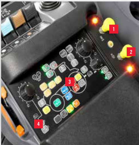
PTO actuation on the Profi and Profi CVT.
