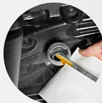
Checking oil level and topping up without lifting the bonnet
