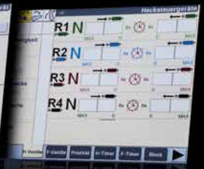
Determine flow rates and time control
