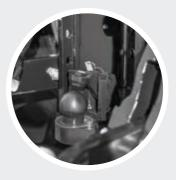
**K80 ball-head coupling**Ideal for heavy-duty trailer operation.
